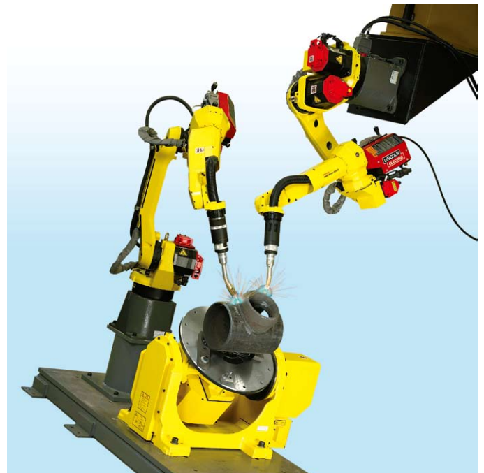
Automobile part arc welding with 2-axes servo positioner
