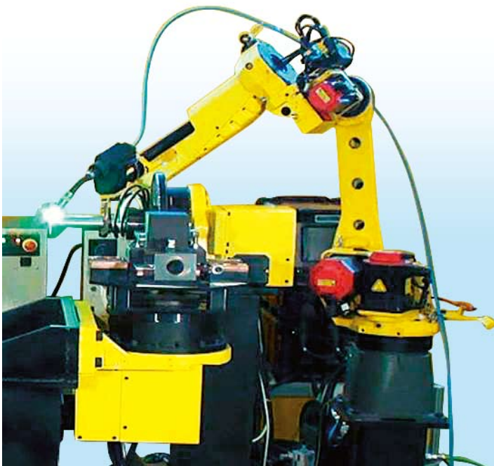
Aluminum part arc welding with 1-axis servo positioner
